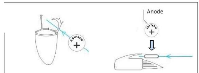
**Note:** 1>after loaded battery, earpiece starts work. 2>Do not load battery in wrong direction.
